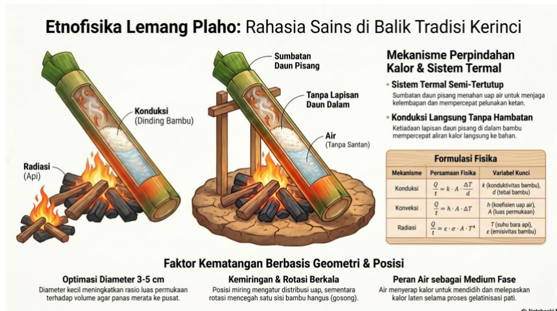
Fig.4. Ethnophysics reconstruction of heat transfer in Lemang Plaho
