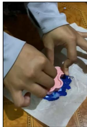
Figure 4. Molding the plastic sheet made from bottle caps using a mold to create the keychain design.
