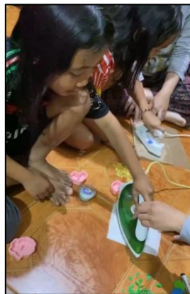
Figure 3. Ironing the cut bottle caps to form a plastic sheet as the base material for the keychain.
